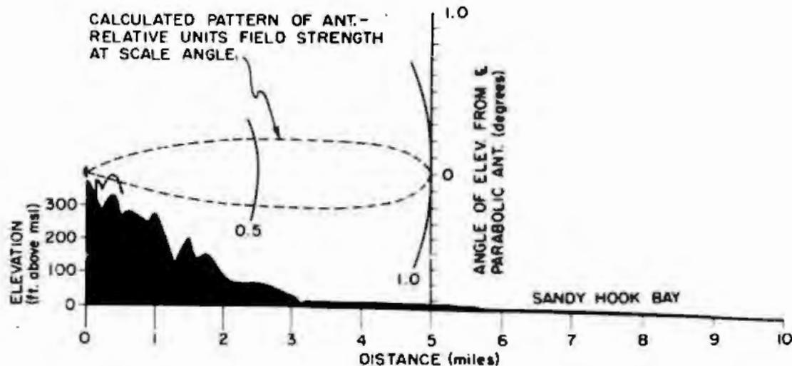
Fig. VI-7. Terrain profile from Crawfords Hill, N. J., along a true bearing of 53° 56' toward Round Hill.
