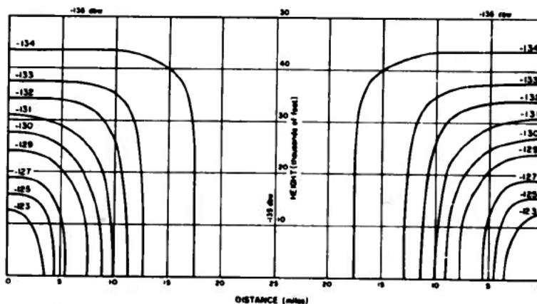
Fig. III-13. Contours of constant reflected signal for 50-mile base.
