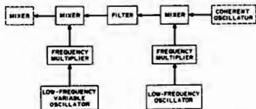
Fig.VC-1. Block diagram of proposed coherent oscillator conversion unit.
