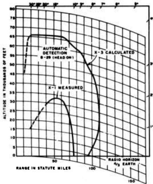
Fig.II-6. Vertical-coverage diagram, Automatic Alerting Radars X-1 and X-3.
