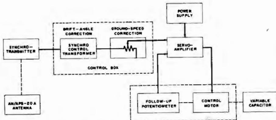
Fig.VC-6. Simplified block diagram of servomechanism drive.
