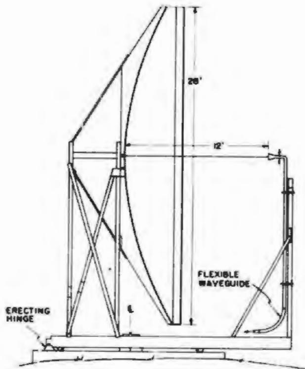
Fig.VI-5. Twenty-eight foot paraboloidal antenna.
