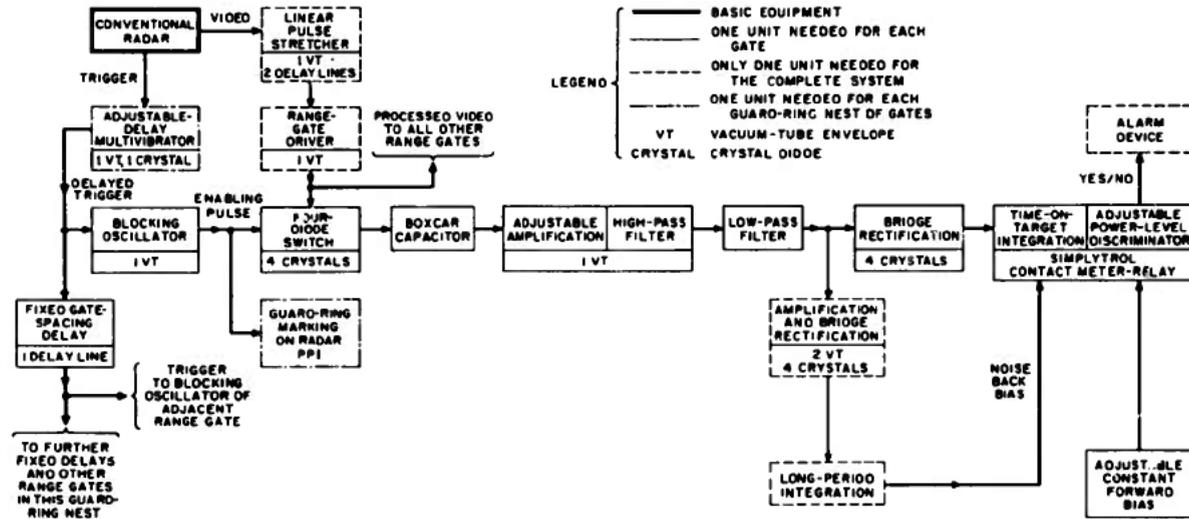
Fig.VF-1. Detailed block diagram of Argus 1, Mk 2.
