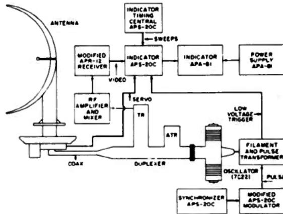
Fig.VG-2. Block diagram of UHF radar.
