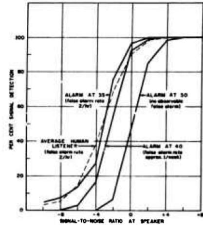
Fig.II-5. Detection by human listener and by alarm at various sensitivities.
