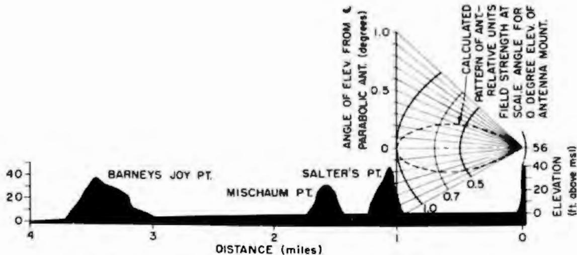
Fig. VI-8. Terrain profile from Round Hill Field Station along a true bearing of 246° toward Crawfords Hill, N. J.
