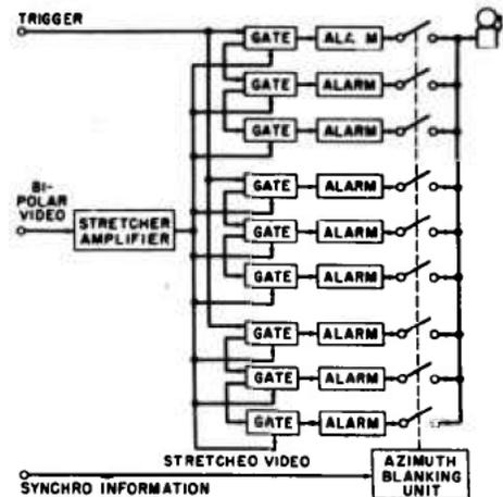
Fig.II-7. Simplified diagram of Radalarm X-3.
