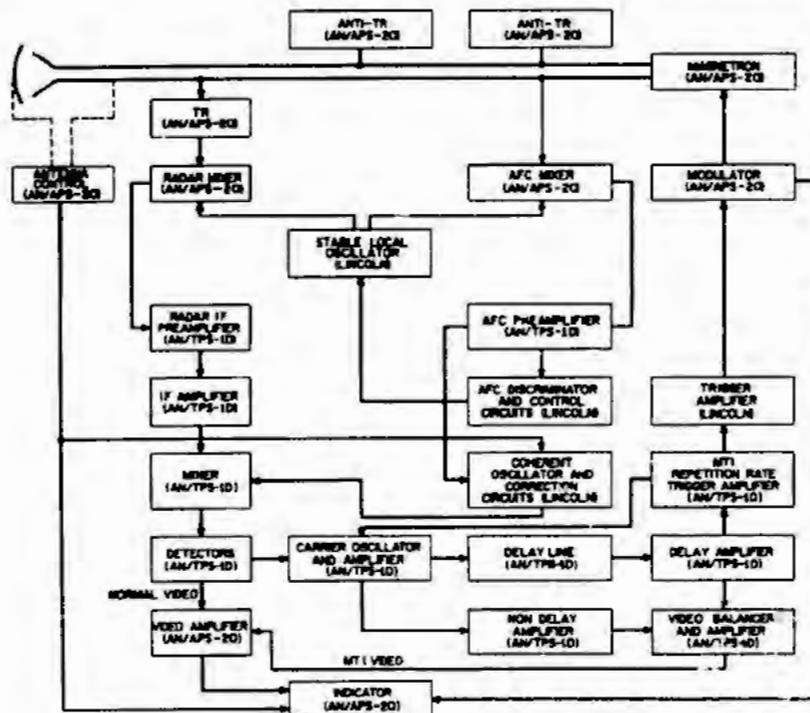
Fig.VC-3. Block diagram of coherent AMTI system.
